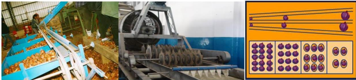
Fig. 3 Sizing onion bulbs by diverging belts/rope
