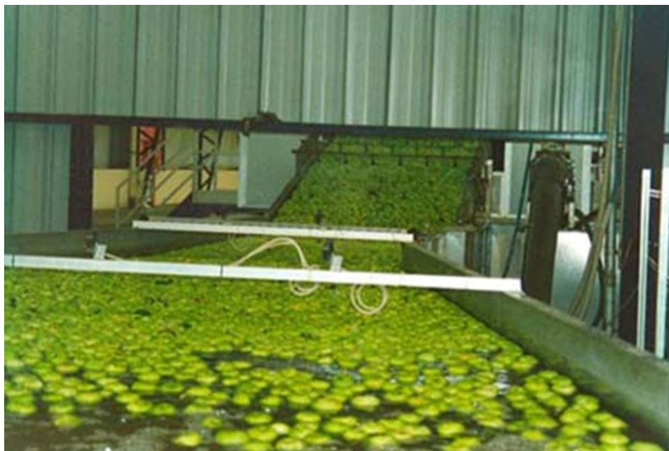
Fig. 2. Water dumping of apples
