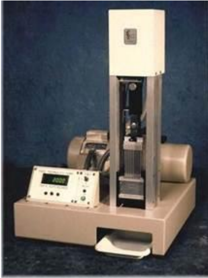
Fig. Tenderometer to test the pea maturity by presser tester
