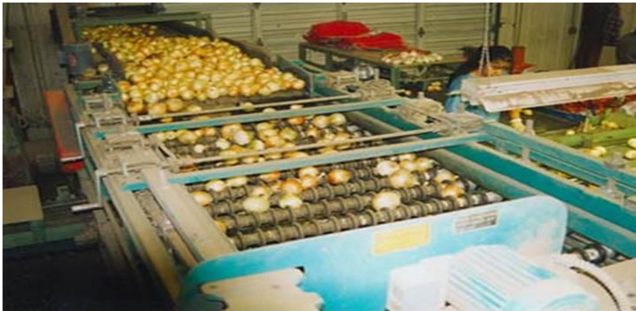
Fig. 4 Sizing by rollers of increasing distance between them
