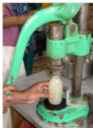
Fig. 1.5: Crown corking machine
