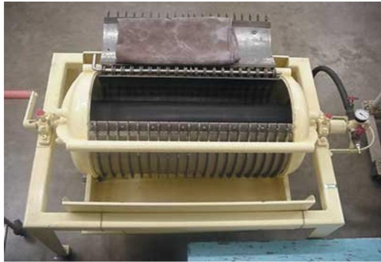
**Figure 1.11: Bladder press, 100L capacity.**
