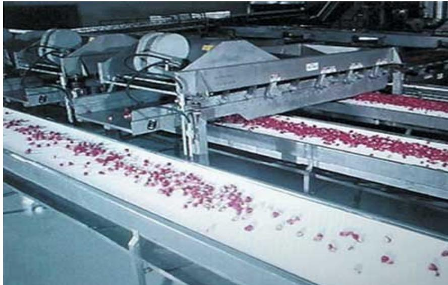
**Figure 1.3: Automatic inspection/grading system.**
