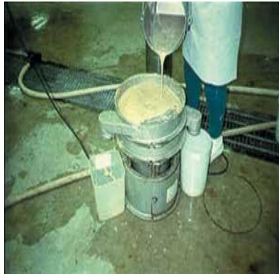
**Figure 1.13a: Shaker separating screen.**
