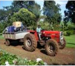
**(b) Row crop tractor:** It is used for crop cultivation. Such tractor is provided with replaceable driving wheels of different tread widths. It has high ground clearance to save damage of crops. Wide wheel track can be adjusted to suit inter row distance.
