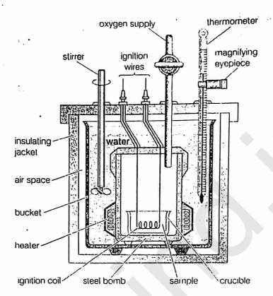
The amount of energy release from the nutrients in bomb calorimeter or oxy calorimeter is known as gross fuel value. 1 g carbohydrate 4.1 Kcal, 1 g fat 9.45 Kcal, 1 g protein 5.65 Kcal
