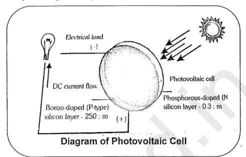
Under peak sunlight conditions a typical commercial PV cell with a surface area of 160 cm<sup>2</sup> will produce about 2 watt peak power. If the sunlight intensity were 40 per cent of peak, this cell would produce about 0.8 watt.
