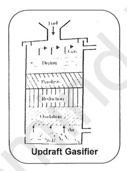
The gas is drawn at higher location. The updraft gasifier achieves the highest efficiency as the hot gas passes through fuel bed and leaves the gasifier at low temperature. The sensible heat given by gas is used to preheat and to dry fuel used.
